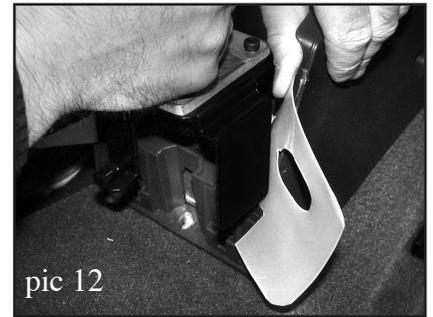
12. Once the base attachment bracket is in the console, press it down so the holes on each side of the base attachment bracket are sandwiched between the 2 metal pillars with the red screw anchors and the center console wall. Be careful not to accidentally knock the red screw anchors off the pillars. Very important: the base attachment bracket must be pushed straight down over the pillars to insure the red screw anchors stay in place. See illustration. (pic 13)
