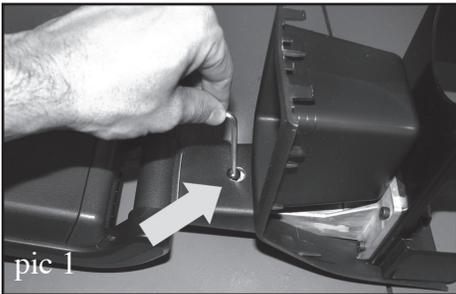
1. Remove the armrest from its packaging. Use 4 mm hex key to loosen the set screw holding the upper armrest assembly to the lower mounting bracket stem. (pic 1) Separate armrest top from lower mounting bracket.
