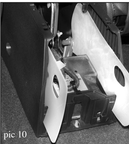
11. Installing the base attachment bracket is the most difficult step of the installation. While lifting the console and spreading the rear opening of the console, insert the base attachment bracket through the rear of the console. The plastic sheets will make the job much easier.
