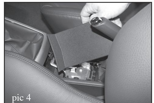
5. Remove the trim piece directly in front of the hand brake. Remove the #20 torx head screw located under this trim piece that secures the front of the console. This will allow the rear of the console to be lifted higher during later steps. (pic 4 & 5)
