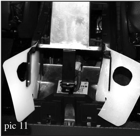
This maneuver is tricky because the rear portion of the base attachment bracket is slightly wider than the opening. It will fit, so don't be afraid to push it in. Be sure to raise the center console sufficiently to clear the tops of the metal pillars with red screw anchors that receive the console screws. (pic 11 & 12)
