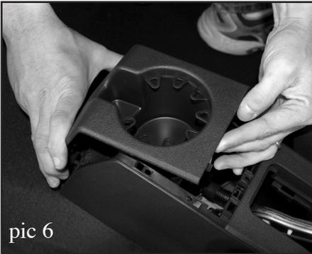
6. After the front edge of the cup holder insert is disengaged from center console, use a pry tool to remove the two nylon trim panel retainers from the bottom rear of the cup holder insert piece and remove the cup holder insert from center console. Put the two nylon trim panel retainers somewhere safe as you will reuse them. The cup holder insert will not be re-used. (pic 6)
