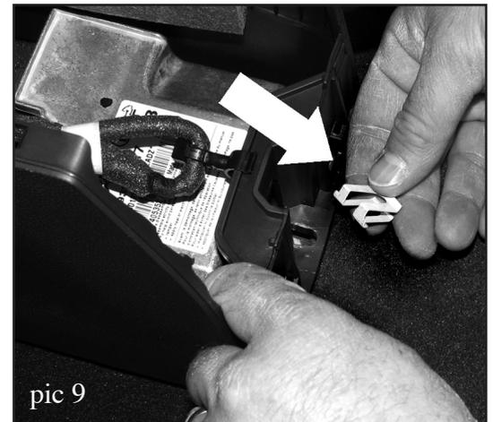
10. Insert the provided plastic sheets on both sides of rear center console as illustrated.
