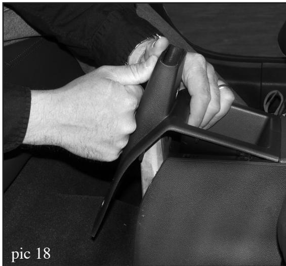
16. Install provided rear bin trim cover insert into rear of center console. This part replaces the rear cup holder which was removed in step #5 and covers the metal armrest stem. Clip the front edge in place
