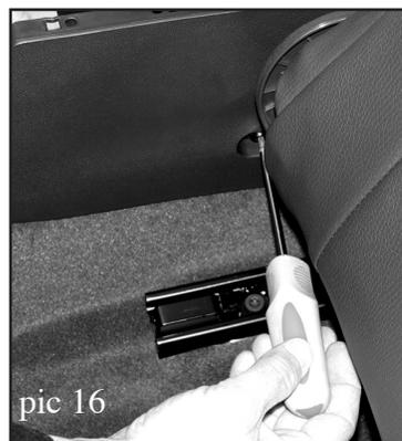
completely tighten at this stage. The rear screws will now secure the center console and the base attachment piece to the steel pillars with the red screw anchors we discussed in step 12. It is very important that both sides align correctly and the screws are reinstalled properly. (pic 15 & 16)
