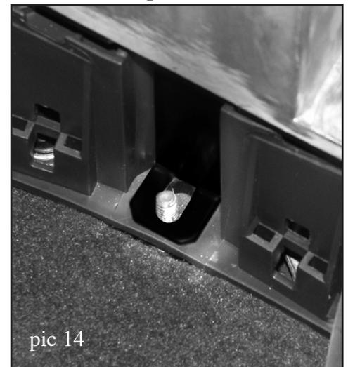
Double check that the metal clip was removed in step #8. (pic 14) When the bracket is properly positioned, remove the plastic sheets.
