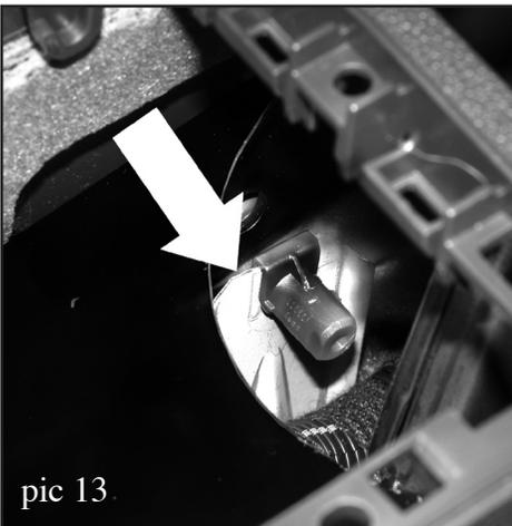
13. Make sure that the tail piece of the base attachment bracket is lined up with the hole in the rear of the center console over the fixed threaded stud.
