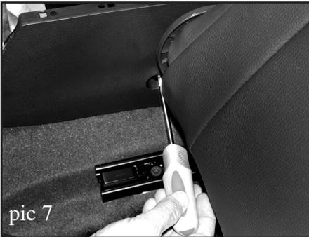
7. Using #20 torx head driver, remove the 2 screws on either side of the rear section of the center console. These screws will be re-installed. (pic 7)
